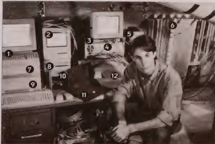
1) FTP server drive. 2) POP mail spooler. 3) Prototype PPP router being tested. 4) Livingston Portmaster router. 5) Norris Earphone atop a stack of modems. 6) punchdown blocks. 7) HTTP server, AURP router, AFP server, PAP spooler. 8) CD drive. 9) mail, FTP, primary nameserver, shell accounts. 10) news spooling drive. 11) Powerbook serves as a mobile administration console, as well as phone book, etc. 12) news and NFS server, secondary nameserver.
